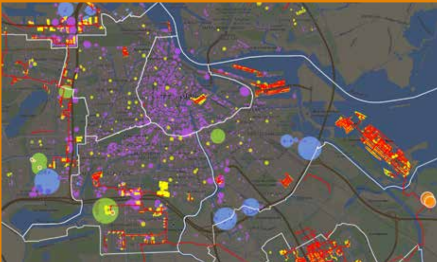
City of Amsterdam, Interactive Maps, 'Energy from waste incineration and waste heat'. The map shows the existing district heat network in Amsterdam (red lines) with connected load (yellow squares) and suppliers of heat (orange circles). The map also shows potential residual or waste heat sources from hospitals (green circles), data centres (blue circles), supermarkets (yellow circles) and offices (purple circles).
